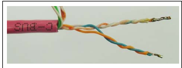
Figure 11 – Soldering may cause cold flow
